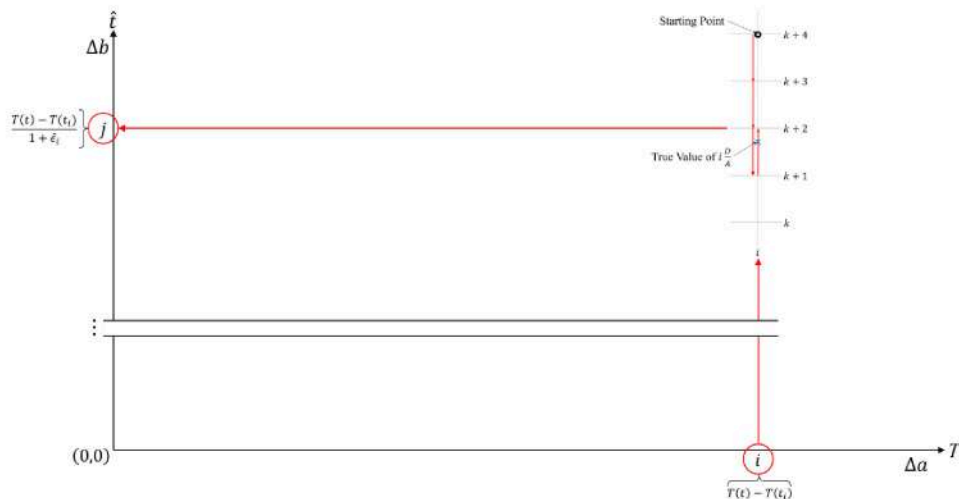
Fig. 5. Sketch of clock skew compensation based on a modified Bresenham's algorithm with vertical
