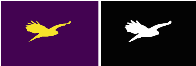
Fig. 5. Mask generation by SAM: 1) left: before dilation-corrosion operation; 2) right: after dilation-corrosion operation
