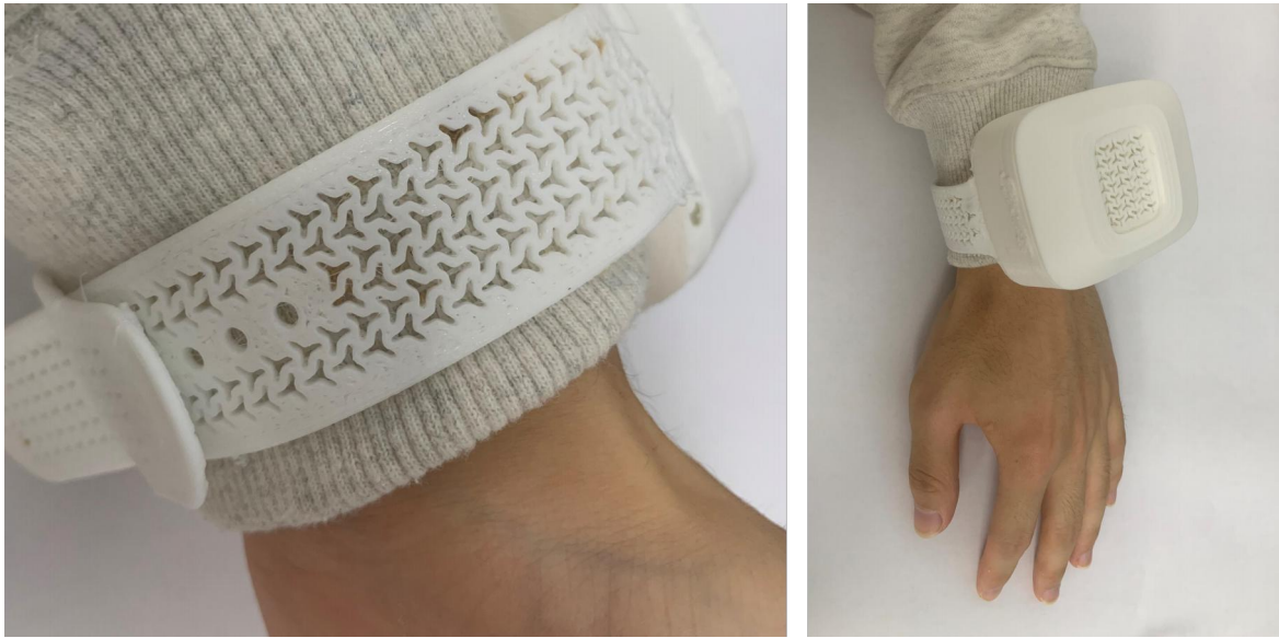
Fig. 4.20 Breathable mesh design for the strap of a wearable device.
