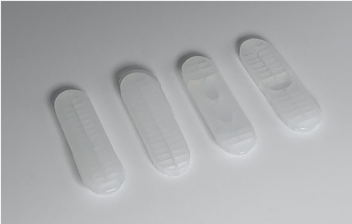
Fig. 4.34 Soft rubber additive manufacturing for soft robot construction moulds.
