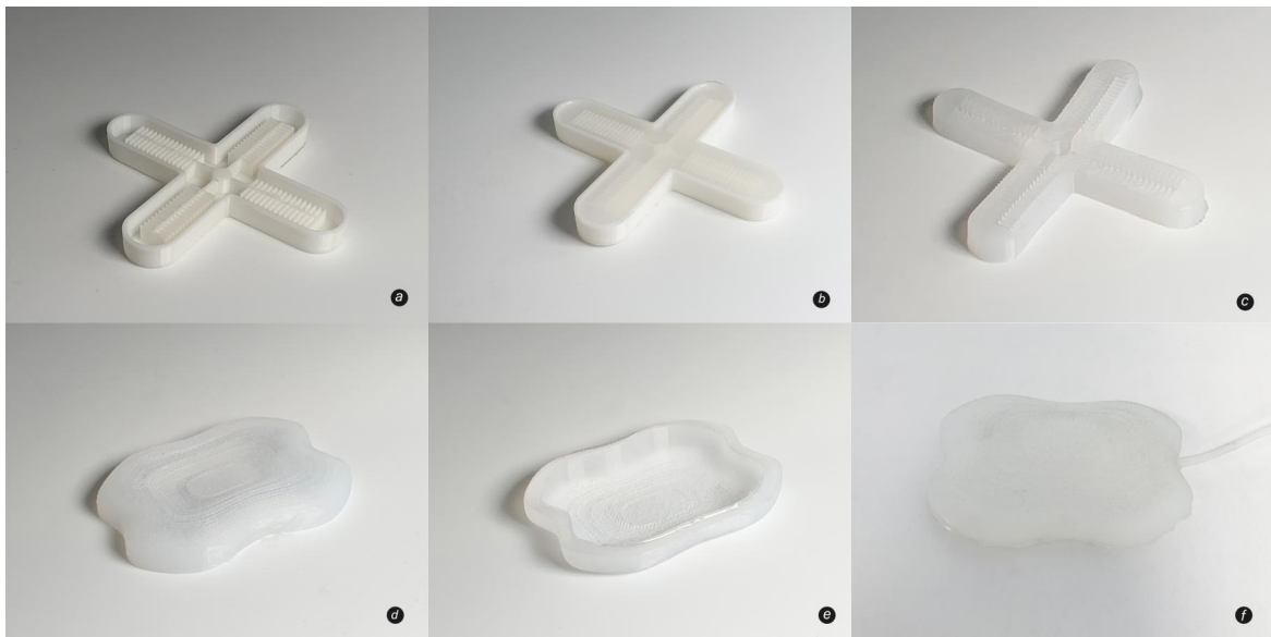
Fig. 4.4 The silicone airbag making process: (a): 3D print the mould (b): introduce the silicone into the mould (c): remove the silicone (d-e): make the front and back silicone (f): combine the silicone and put in the hose
