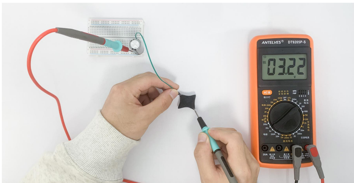
Fig. 4.29 Testing the electrical conductivity of silica materials incorporating highly reactive carbon nanotube.
