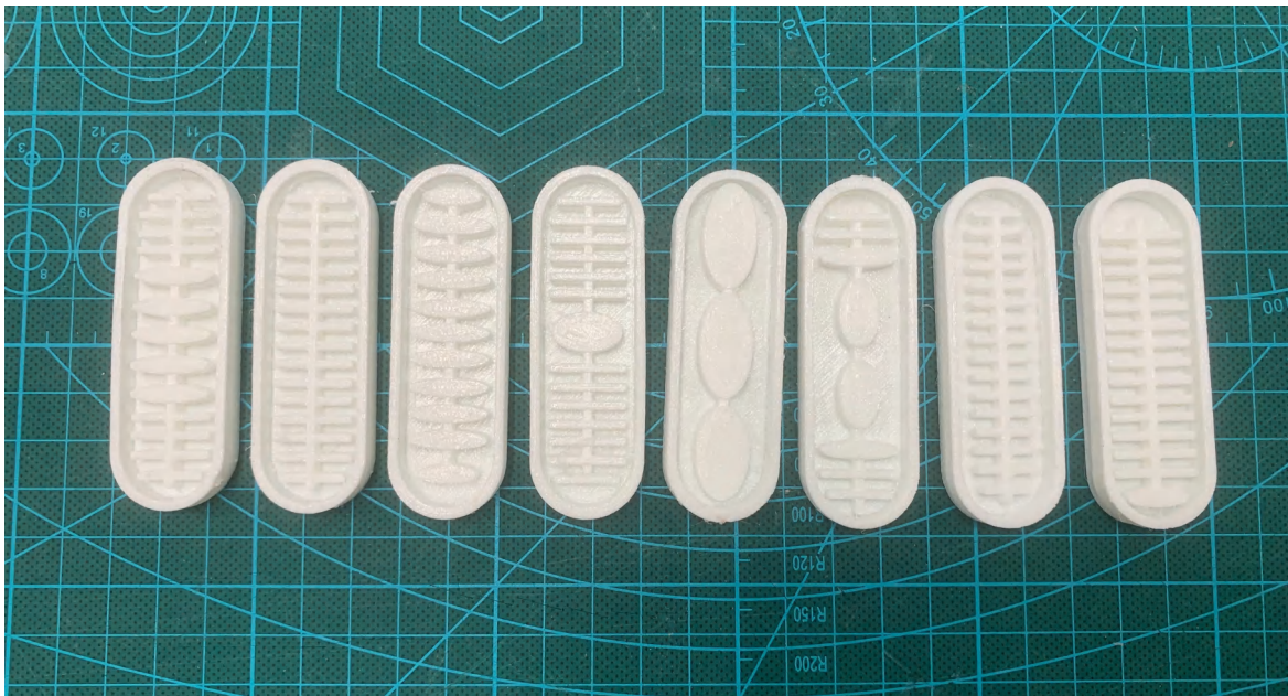
Fig. 4.33 Soft rubber additive manufacturing for soft robot construction moulds.
