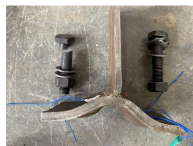
(c) Specimen S-F12-B10.9-P0, a mixed mode
