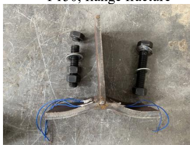
(b) Specimen S-F10-B10.9-P150, flange fracture
