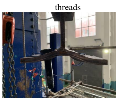
(j) Specimen D-F12-B12.9-P175, bolt fracture
