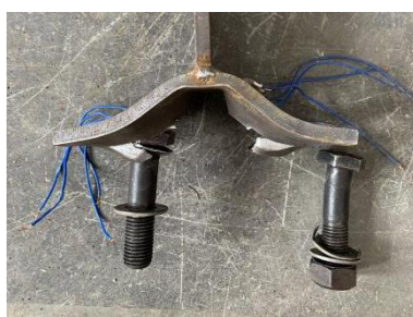
(b) Specimen S-F10-B10.9-P150, flange fracture
