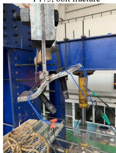
(h) Specimen D-F12-B10.9-P0, stripping of the nut
