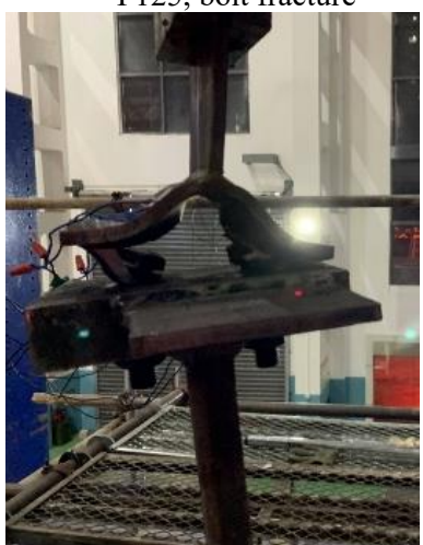
(g) Specimen D-F10-B10.9-P150, flange fracture
