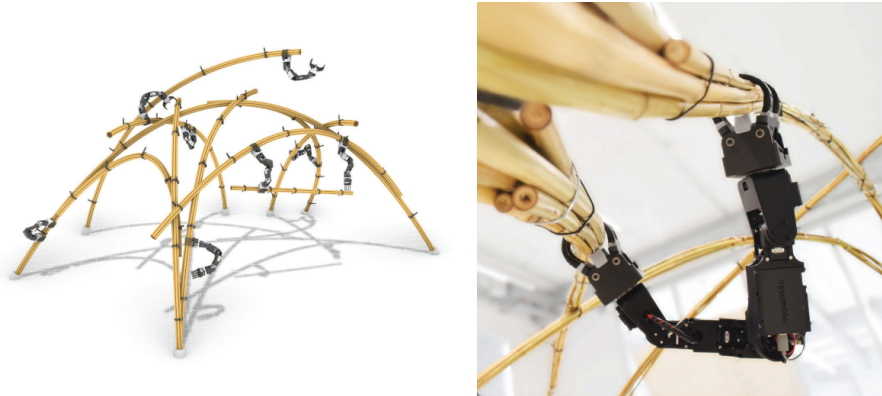
Figure 15. Mobile robot prototypes used in feasibility studies assemble lightweight bamboo bundle structures (Lochnicki et al., 2021)
